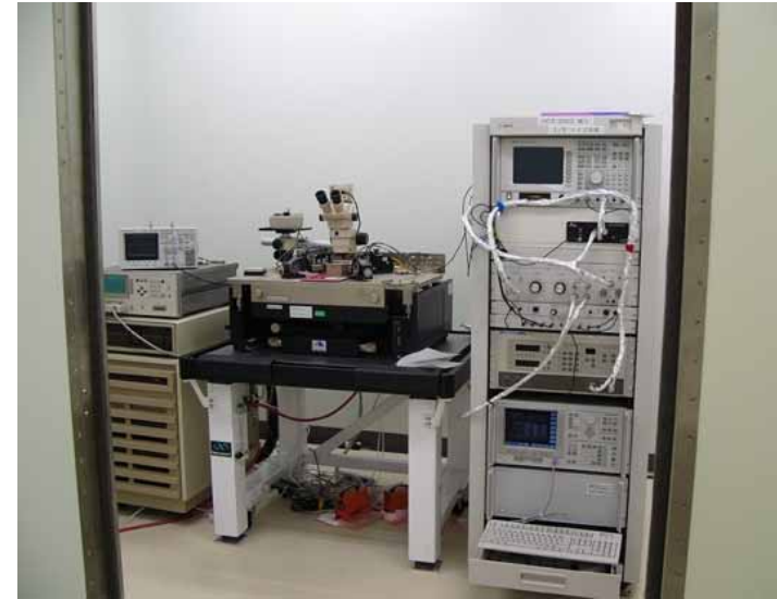
1/f noise measurement system; 6 inch wafer
